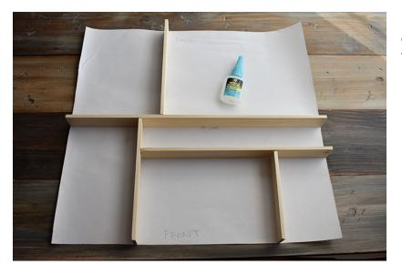
Use your paper template to decide how long to cut each board. Don't forget to include the thickness of the boards in your final measurement when you have perpendicular pieces!
